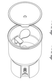
5. Plug the head of power adaptor into the power jack at the bottom of base and plug the power adaptor into the wall socket.
